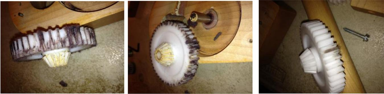
These first 2 photos show an extremely filthy situation. This unit was basically “locked up” and could no longer operate until it was cleaned out. The one on the right was pretty clean except shortly after it was cleaned a clump of yarn got inside. This resulted in a “clunking” sound every time it went around.
